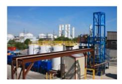
Tradebe's vacuum-assisted Thin Film Evaporator, a wiped film evaporator, is a process that separates volatile from less volatile components using indirect heat transfer and mechanical agitation.
